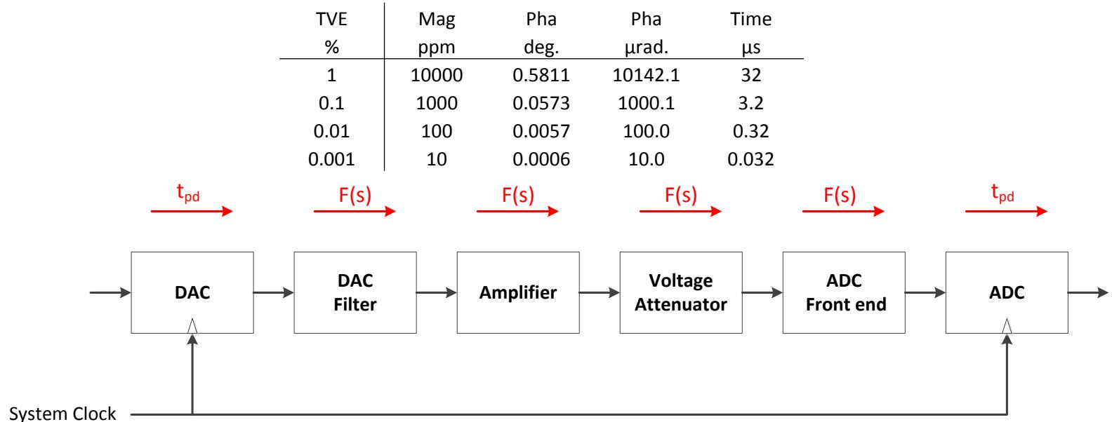
**Impact of Amplifier Bandwidth 6.5 kHz (Single Pole model)**
